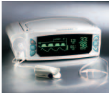
Quiet System monitors ETCO 2 and SpO 2 without disturbing sleep study patients.
